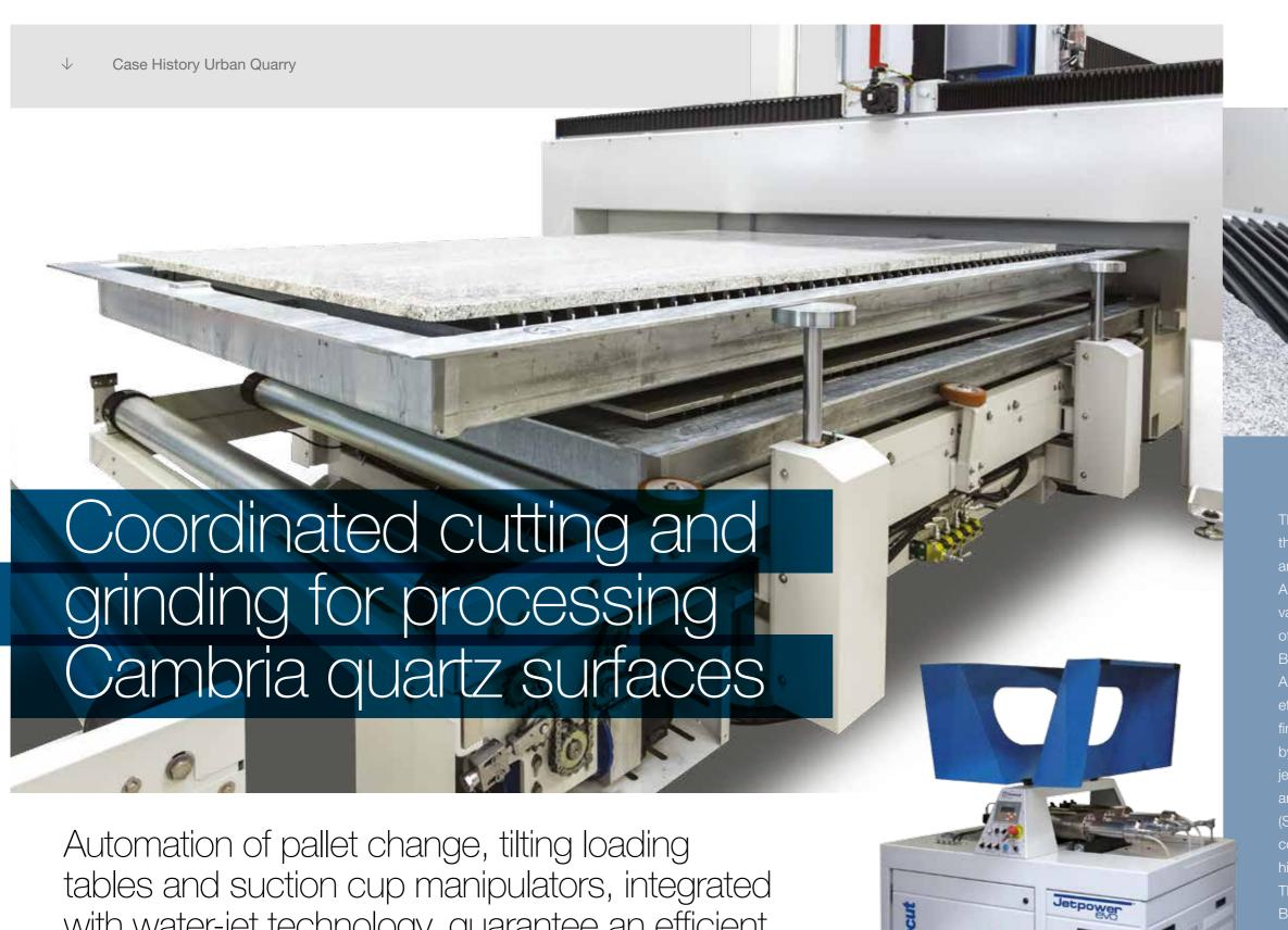
Automation of pallet change, tilting loading tables and suction cup manipulators, integrated with water-jet technology, guarantee an efficient productivity, able to continuously feed the grinding and drilling department. Highest quality finishing and reliability thanks to the 4 CMS Brembana working centres.
